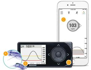
C. <u>Display Device</u> - Receives and displays sensor glucose levels. This must be within 20 feet of the sensor in order for information to be received. This can be your own mobile device or a manufacturer-issued receiver.
